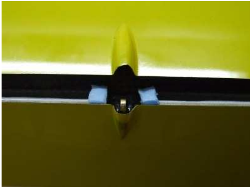
Glue horn with thickened epoxy.
