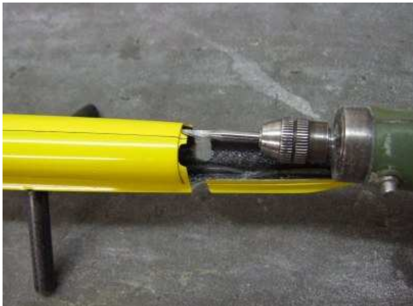
Reduce wall thickness of fuselage laminate where they move to gain space.
