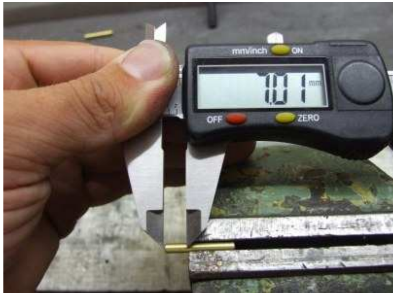
Bending the rudder horns from brass tube OD=3, ID=2, L=21 mm.
